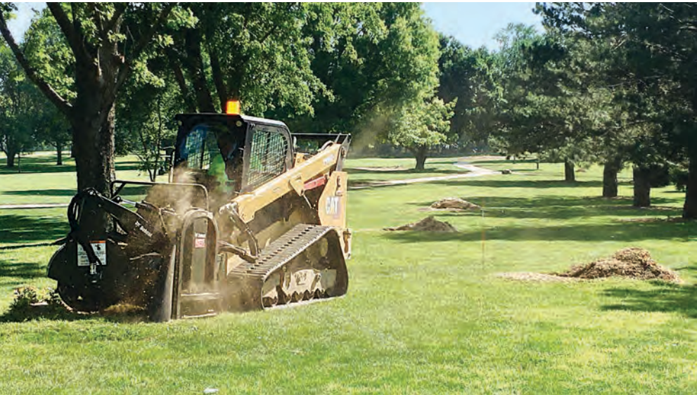
Mike Monthei, LPA maintenance supervisor, operates a stump grinder attached to a skid loader to remove one of 304 stumps left behind when ash trees on the Lake Panorama National course were removed. Work on this long-term project began July 20 on the first hole of the LPN golf course. In the background, mounds of mulch residue can be seen where three other stumps had already been removed.
