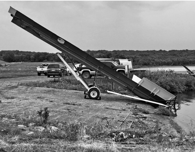
Once the skimmer is filled with debris, it backs up to the elevator shown here. A conveyor belt on the elevator moves the debris upwards to be deposited into dump trucks.
