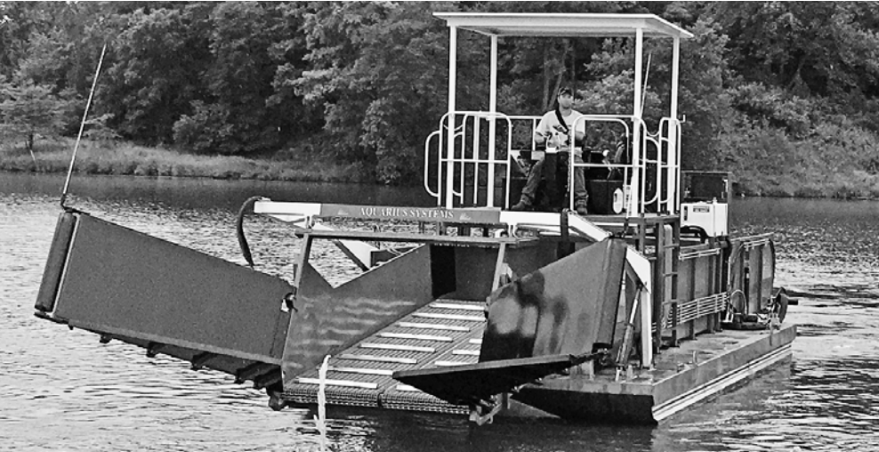
An employee of Aquarius Systems was on hand to demonstrate how the debris skimmer operates. This view shows the front gates open and the conveyor belt, which work together to scoop up debris and move it to a storage area in the back of the skimmer.
