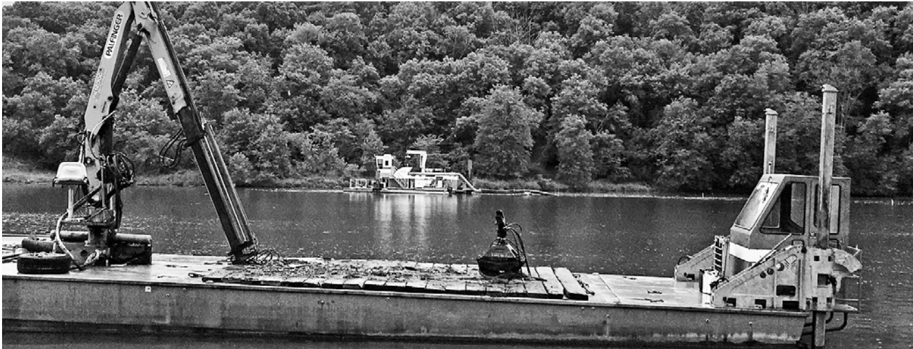
Shown here is the utility barge purchased in 2009 by RIZ and the LPA. A boom mounted on the barge accommodates a grapple attachment to remove logs from the water. Shown beyond the barge is LPA's dredge, which has been working through the summer in the Middle Raccoon River above the debris trap.
