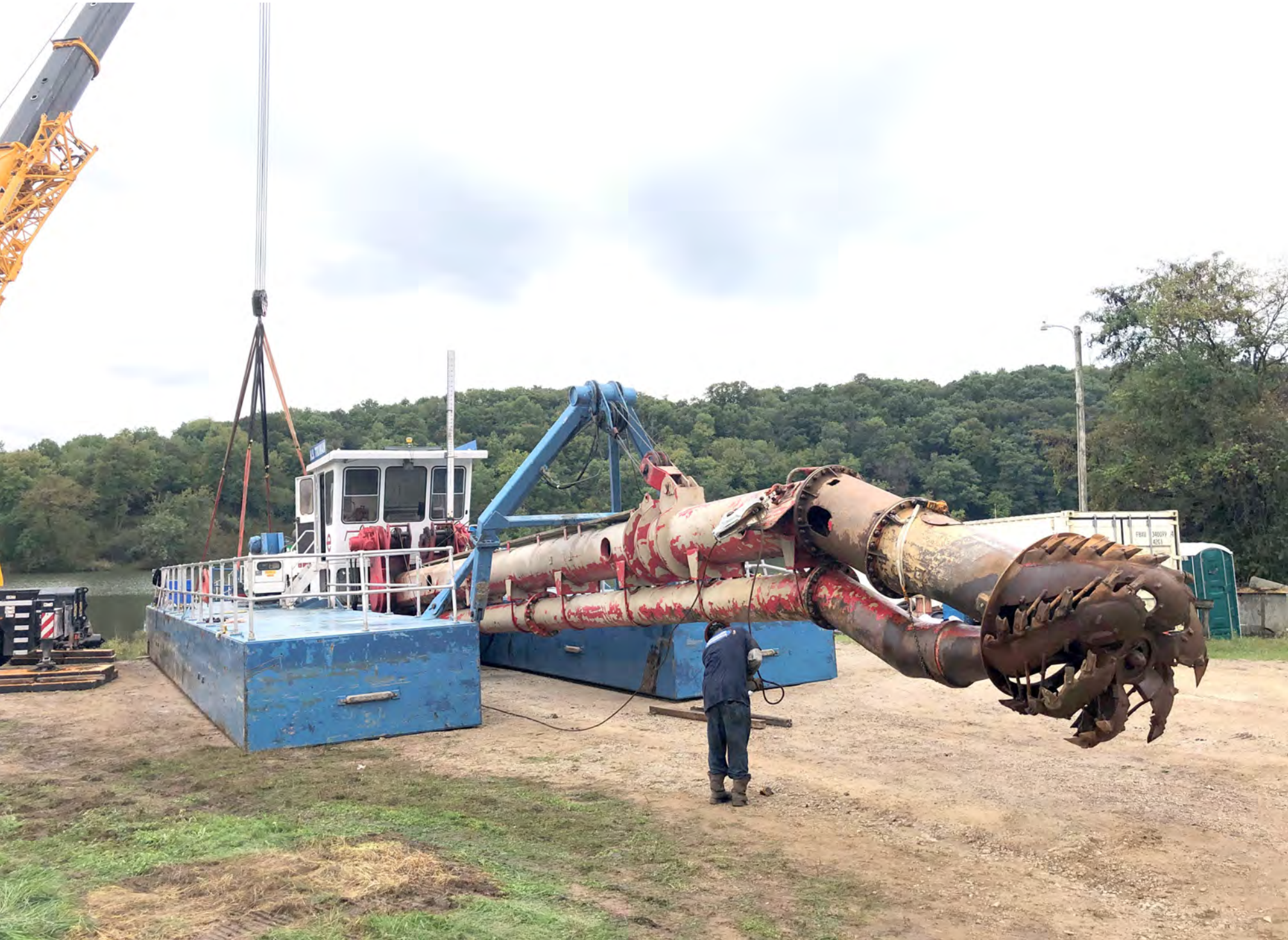
A Dredge America employee is shown working on the dredge's cutter head on land north of Lake Panorama's upper basin.
