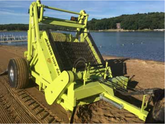
The groomer features tines on a moving belt. As it is pulled along the sand, the tines pick up goose manure, sticks and other debris, which drop into a hopper on the back.
